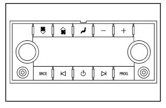
$\overset{}{\bigcup}$  (Power): Press the  $\overset{}{\bigcup}$  button to turn the RSA on or off.
